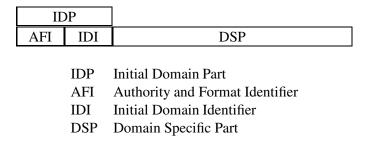
Figure 3: NSAP address structure.
